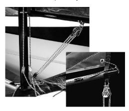
Unpack the jib and to its top fix the lifting rope. Then pull up the jib and its bottom corner with the jib furler fix with a carbine as shown on the photo below. Roll out the mainsail and attach the lifting rope running from the top of the mast to it. Insert the sail in the notch in the mast and pull the lifting rope to lift it up. Then tie up the rope to the sling on the mast.
