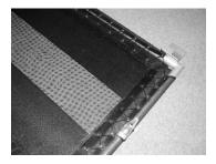
Fix the keel fins on the bottom of the non-inflated floats. Push the fins into the pockets on the floats.
