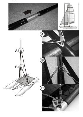
Now you can erect the mast. By tightening the front rope and locking it in the notch you can achieve thorough tautening for all the ropes and the mast. Screw in the stretchers on the lower stainless ropes in such a manner so that these are tautened.
