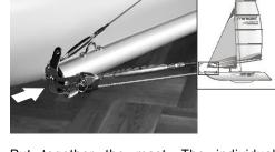
Put together the mast. The individual components are just put in one another. Interlace the lifting ropes with a pulley on the top of the mast. Before erecting the mast, fix the lateral fastening ropes in its upper part as well as the front rope. Attach the other ends of lateral guy-ropes to the frame using shackles. Attach the front rope to the snap hook on the longitudinal centre tube.
