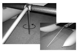
Unwrap the bundle of stainless ropes and attach them using snap hooks to the frame as shown in the diagram. Slip the end with a plastic plug on the end of the longitudinal centre tube.
