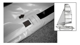
Attach the frame to the non-inflated floats. Attach the frame by pushing the flags into the pockets on the floats.
