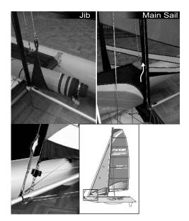
Lace the foresheets through the grommets on the frame and tie a knot to prevent them from pulling out.
