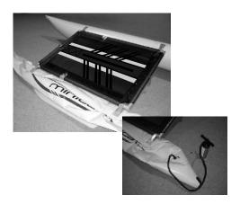
Before inflation, check the status of the valves. Set the valves to the closed position, slightly push on the centre pin, turn the pin and release the pressure on the pin to enable it to sit in the higher position.
