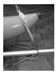
Unpack the jib and to its top fix the lifting rope. Then pull up the jib and its bottom corner with the jib furler fix with a carbine as shown on the photo below. Roll out the mainsail and attach the lifting rope running from the top of the mast to it. Insert the sail in the notch in the mast and pull the lifting rope to lift it up. Then tie up the rope to the sling on the mast.
